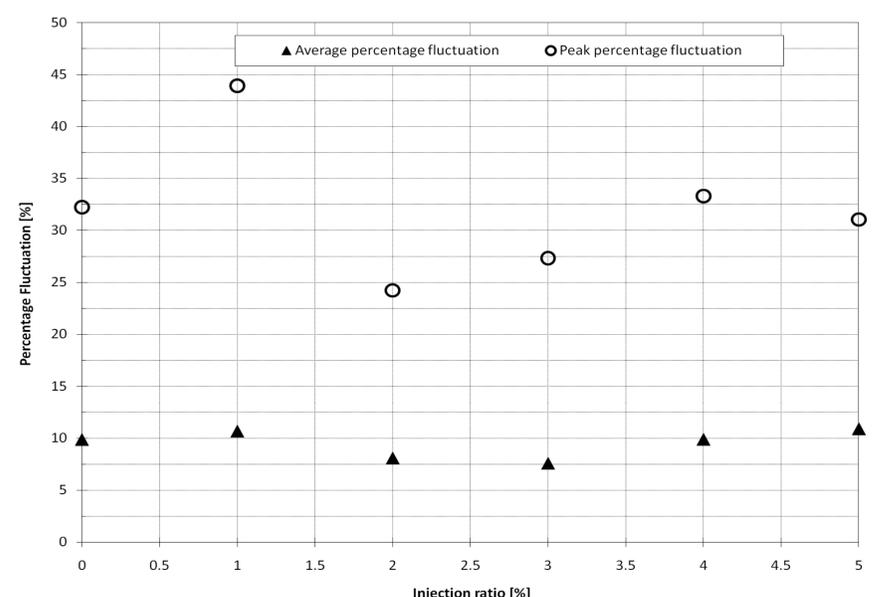
Fig 3: Percentage pressure drop fluctuation as a function of injection ratio for a perforated tube with seven perforation holes, which are equi-spaced around the circumference of a tube and a pitch-diameter ratio of 0.75
