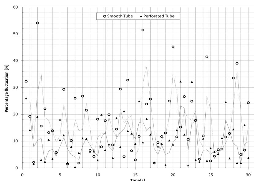
Fig 2: Percentage pressure drop fluctuation from the mean pressure drop under turbulent conditions across smooth and perforated tubes using a centrifugal pump to drive the flow
