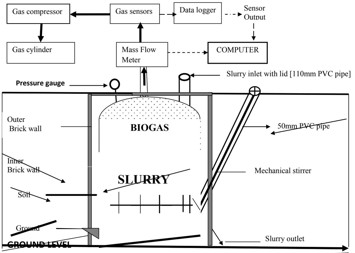
Figure 1. Schematic diagram of the experimental set-up of a batch field biogas digester
