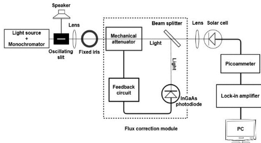
Figure 1: Schematic diagram of the differential measurement setup using feedback response module.
