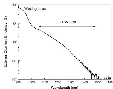
Figure 4: External quantum efficiency spectrum of the GaSb/GaAs quantum ring solar cell
