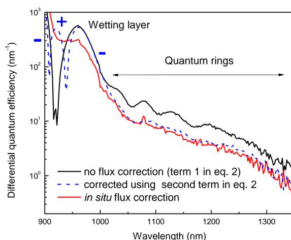
Figure 5: Differential photocurrent spectrum of the GaSb/GaAs quantum ring solar cells, with and without in situ flux correction. The +/- signs represent the phase of the signal.
