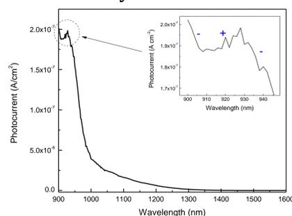
Figure 2: Photocurrent spectrum measured for the GaSb/GaAs quantum ring solar cell. The inset highlights the change in slope near the GaAs band edge.
