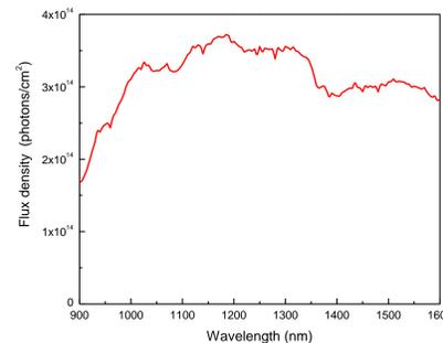
Figure 3: Spectral dependence of the photon flux used for the response measurements.
