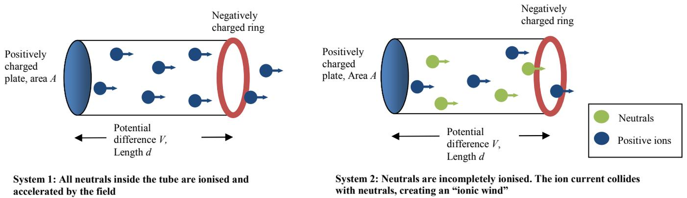
**Figure 2.** Description of system 1 and system 2, as used in the derivation (see text)
