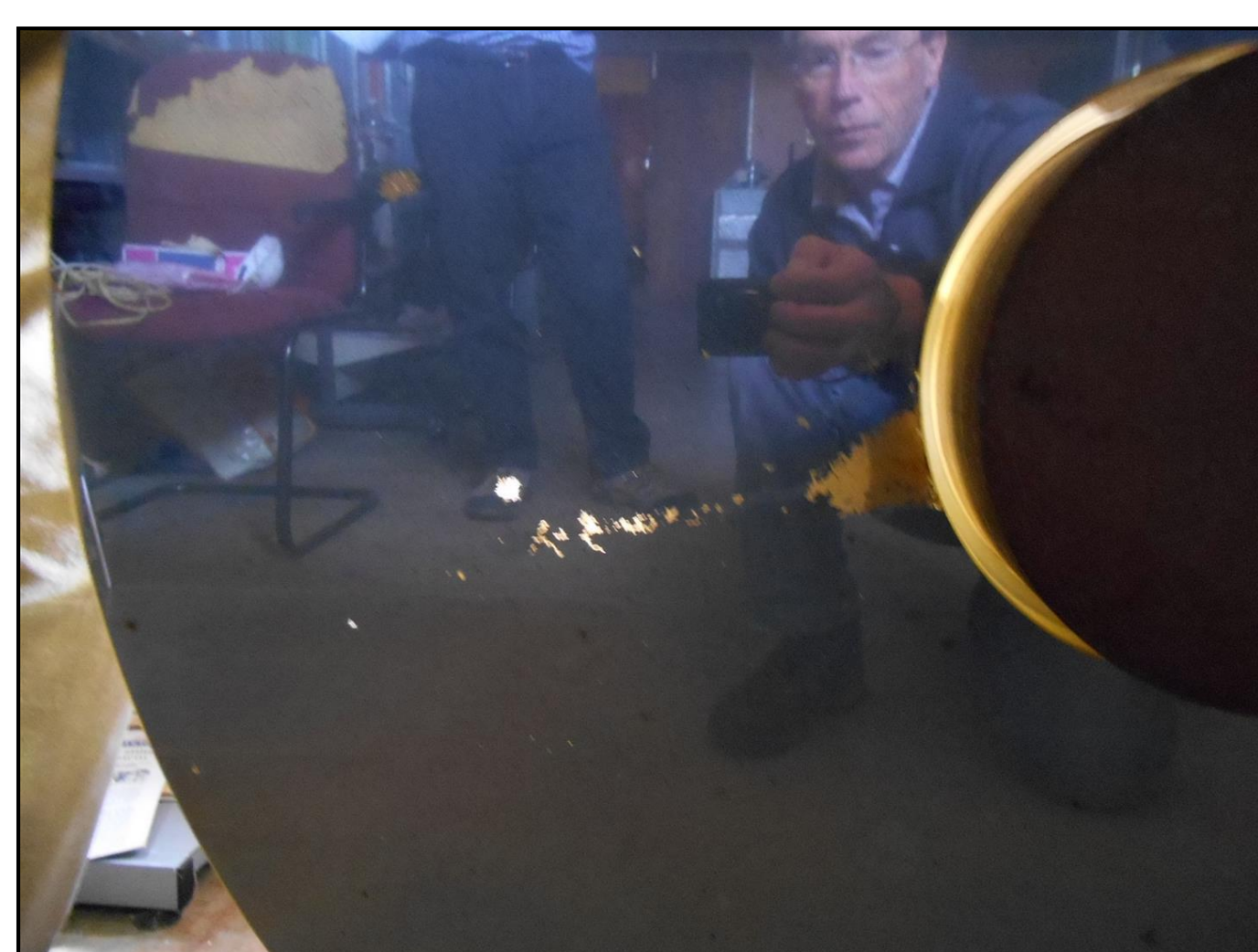
Figure 3: Coating degradation on primary mirror.
