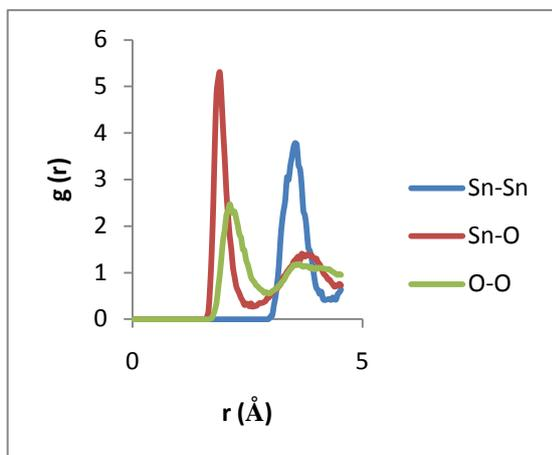
Figure 1 pair correlation function for rutile tin-oxide at 400 K.
