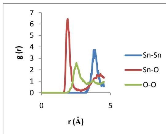
Figure 2 pair correlation function for rutile tin-oxide at 900 K.
