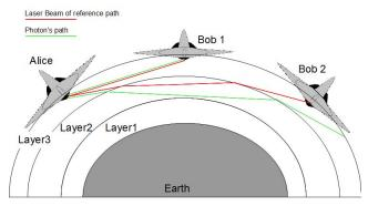
**Figure 4.**Different conditions of link for atmospheric vehicle. The picture show that the path of laser change if the vehicle are the same altitude. This phenomena occur by the curve of the Earth.
