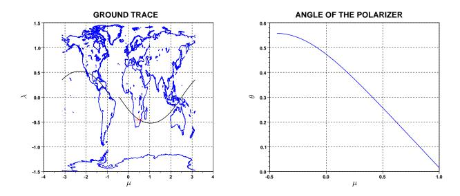
Figure 2. Angle of polarizer  $\theta$  in function of the longitude  $\mu$ . It is possible to observe from the first chart the simulation which considers the satellite that crosses the geographical position of Johannesburg.
