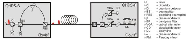
**Figure 3.** Clavis<sup>2</sup> QKD system from id Quantique.
