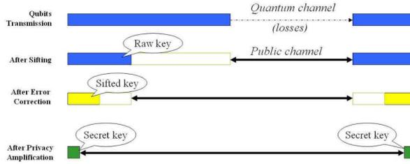
**Figure 1.** Key generation stages in BB84 protocol. An image courtesy of [4].
