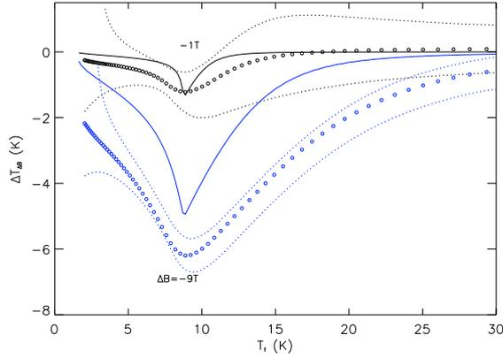
**Figure 3.** The adiabatic temperature change  $\Delta T(T_f)_{\Delta B}$  calculated from the isofield entropy curves in figure 1 for  $\Delta B = 1$  T and 9 T (open circles). Dotted lines show the uncertainty in the calculation. Solid lines show the adiabatic temperature change calculated for the corresponding mean field ferromagnetic system.
