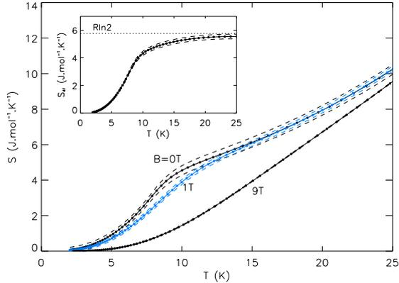
**Figure 1.** The isofield entropy (filled circles) for CeAuGe calculated from experimental specific heat data in zero field, 1 T and 9 T. Upper and lower bounds are indicated by dashed lines. Inset: Magnetic configurational entropy of the  $\text{Ce}^{3+}$  4*f*-electrons in CeAuGe in zero applied field.
