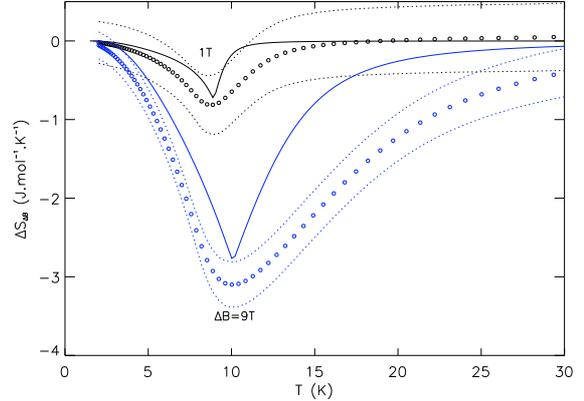
**Figure 2.** The isothermal entropy change  $\Delta S(T)_{\Delta B}$  (open circles) calculated from the isofield entropy curves in figure 1 for  $\Delta B = 1$  T and 9 T. Dotted lines show the uncertainty in the calculation. Solid lines show the isothermal entropy change calculated for the corresponding model mean field system.
