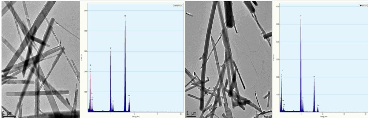
**Figure2.** High magnification Transmission electron microscopy images and elemental composition of VO<sub>2</sub> as-synthesized and anneal nanoplatelets.
