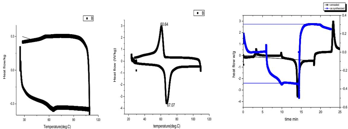
**Figure3.** DSC curve showing the reversible phase transformation in the material during the thermal cycling in as synthesized material VO<sub>2</sub>(A) and VO<sub>2</sub>(M) and kinetics effects of both samples.
