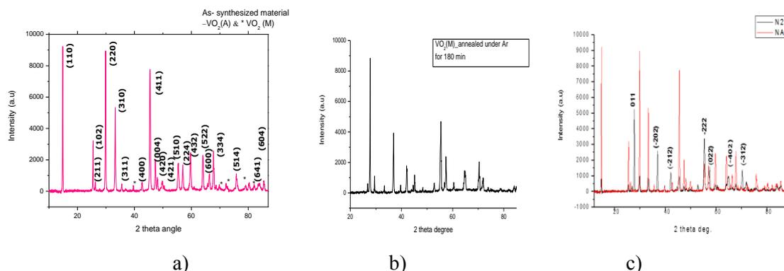
**Figure 5.** Typical room temperature indexed X-rays diffraction of the as-synthesized a) annealed under Argon b) and annealed under Nitrogen c) nanostructures materials.
