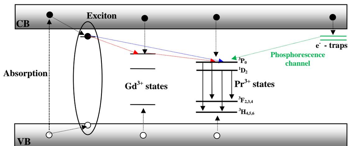
**Figure 6:** The phosphorescence and energy transfer mechanism
