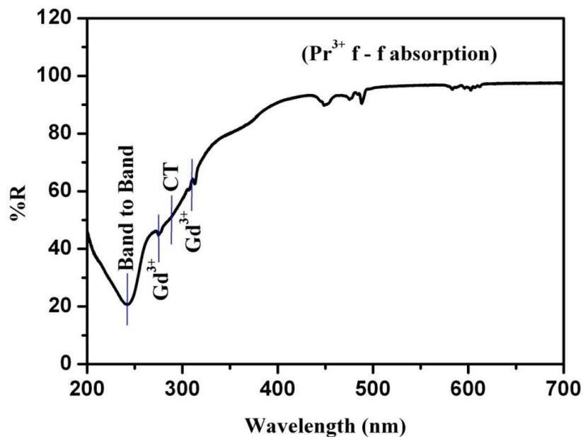
**Figure 3:** Diffuse reflectance spectrum of  $\text{GdTaO}_4:\text{Pr}^{3+}$
