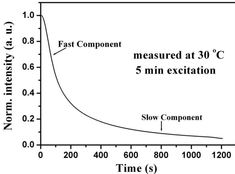
**Figure 5:** The phosphorescence lifetime spectrum measure at 30 °C
