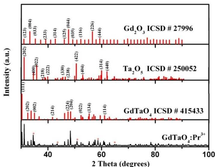
**Figure 1:** XRD patterns of  $\text{GdTaO}_4:\text{Pr}^{3+}$
