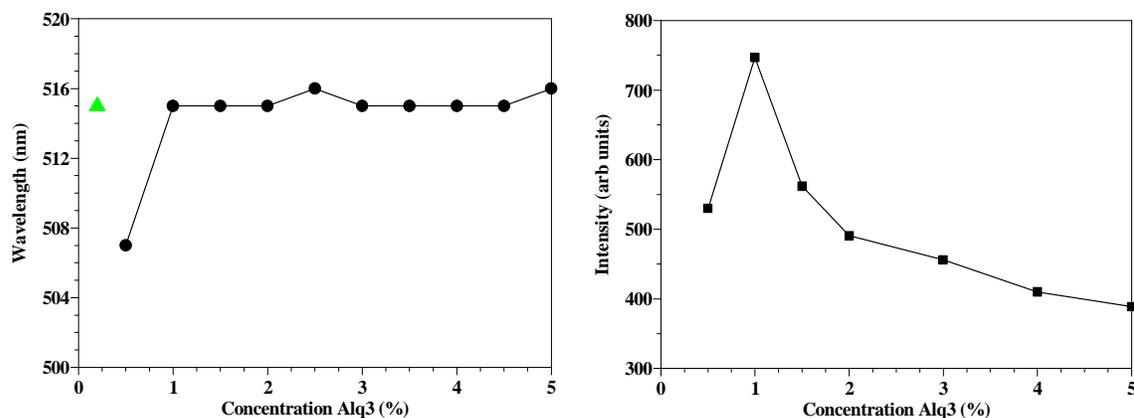
Figure 4: (a) A plot of the emission wavelength at maximum intensity as function of the Alq<sub>3</sub> concentration. The triangle represents the emission of Alq<sub>3</sub> in the solid state. (b) Plot of PL maximum intensity as a function of concentration of Alq<sub>3</sub>.
