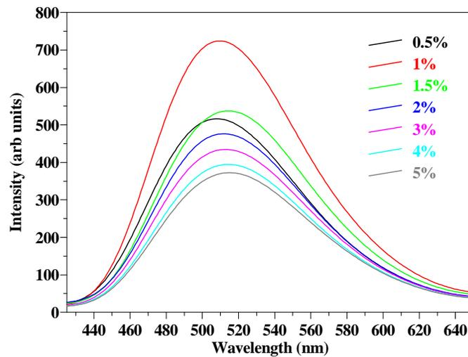
Figure 3: Photonluminescent spectra of different concentrations of Alq<sub>3</sub> in a PMMA matrix, just after synthesis.
