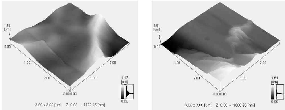
Figure 2: AFM images of two different spots on the 1% Alq<sub>3</sub>:PMMA film.
