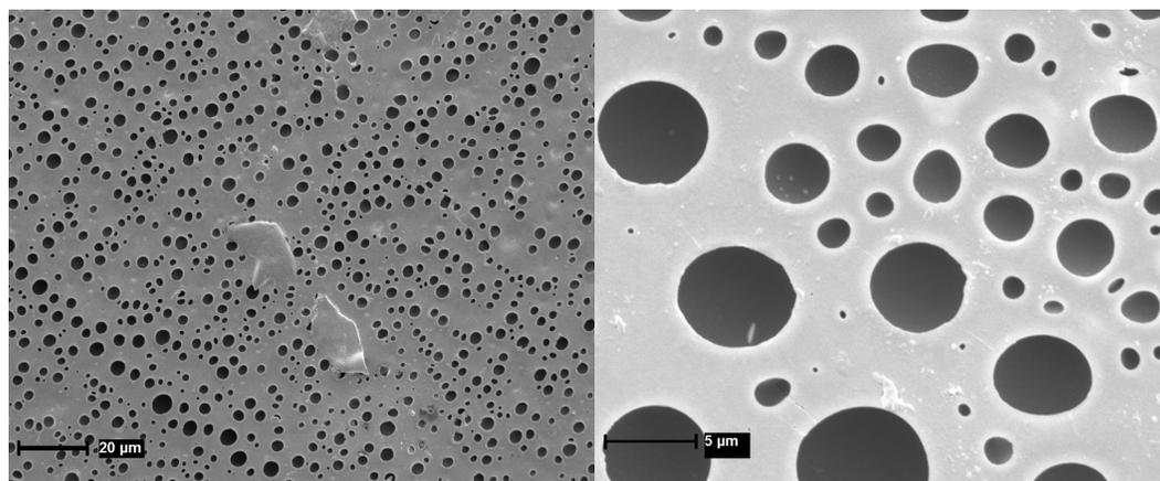
Figure 1: SEM images of 1% Alq<sub>3</sub>:PMMA at x1000 and x5400 magnifications. Holes that had formed during the evaporation of the solvent can clearly be seen.
