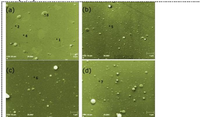
**Figure 3.** SEM images, for the thin film surfaces, grown in (a) base, (b) O<sub>2</sub>, (c) Ar and (d) N<sub>2</sub> pressure.
