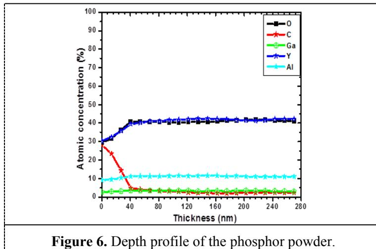
**Figure 6.** Depth profile of the phosphor powder.
