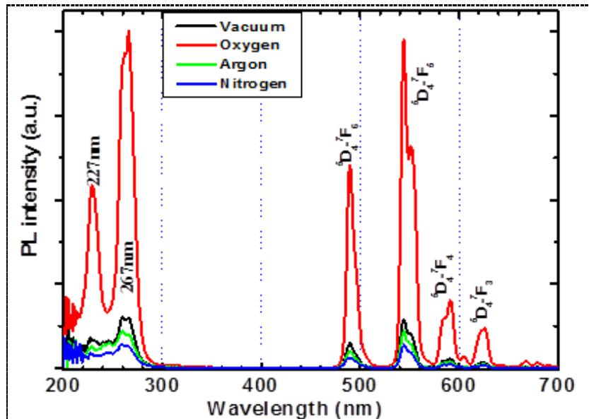
**Figure 7.** PL emission and excitation of  $Y_3(Al,Ga)_5O_{12}:Tb$  thin films grown in different working atmosphere (Excitation measured at an emission wavelength of 544 nm; emission measured at an excitation wavelength of 267 nm).
