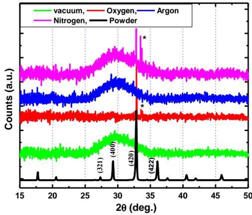
**Figure 1.** XRD spectra of Y<sub>3</sub>(Al,Ga)<sub>5</sub>O<sub>12</sub>:Tb phosphor powder and thin films grown in different working atmosphere.
