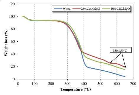
Figure 1: Thermal degradation of wood and blends at the heating rate of 20°C/min
