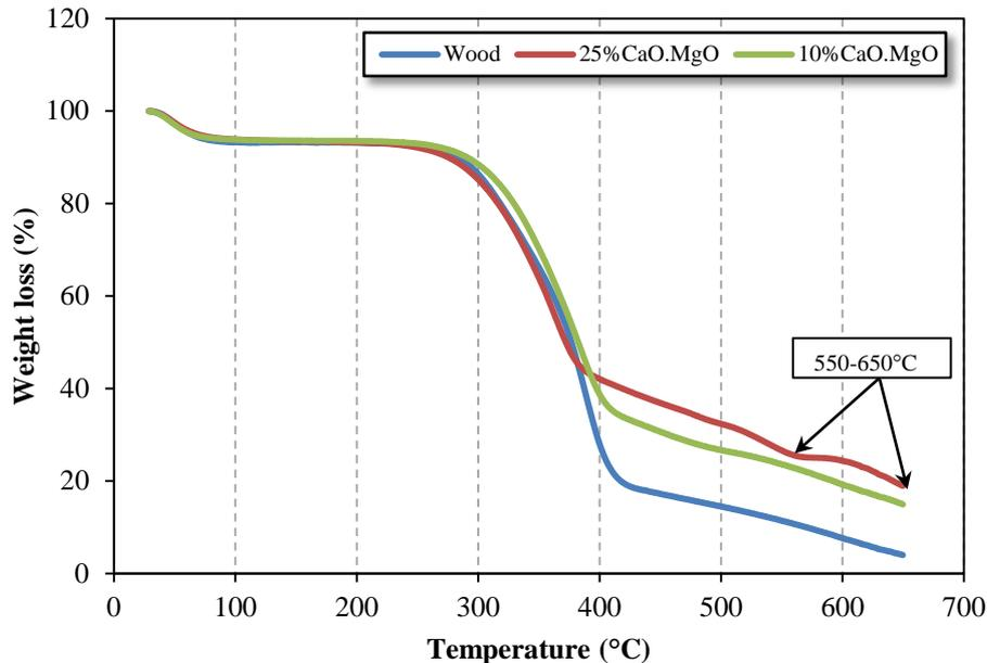
*Figure 1:* Thermal degradation of wood and blends at the heating rate of  $20^{\circ}\text{C}/\text{min}$
