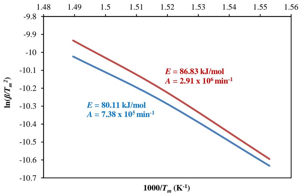
**Figure 3:** Plots of  $\ln(\beta/T_m^2)$  versus  $1000/T_m$  of wood sample (blue plot) and 25% CaO.MgO blend (red plot) for the heating rates of 10°C/min, 15°C/min and 20°C/min
