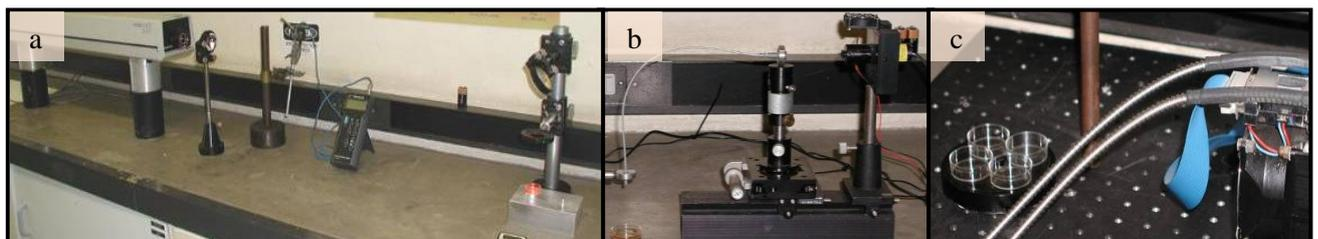
**Figure 1.** Laser irradiation of cells using a He-Ne laser (a), 830 nm diode (b) and Nd:YAG laser (c).
