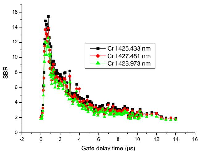
**Figure 1.** Effect of gate delay time variation on signal-to-background ratio of Cr I lines of soil sample.
