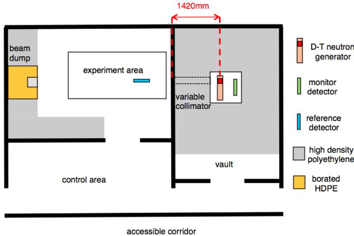
**Figure 1.** Layout of the fast neutron facility at UCT. The generator is installed within the vault, surrounded by HDPE shielding. Neutrons enter the experimental area via the variable collimator. Detector and generator controls are located in the control area. All areas are access controlled unless explicitly labelled.
