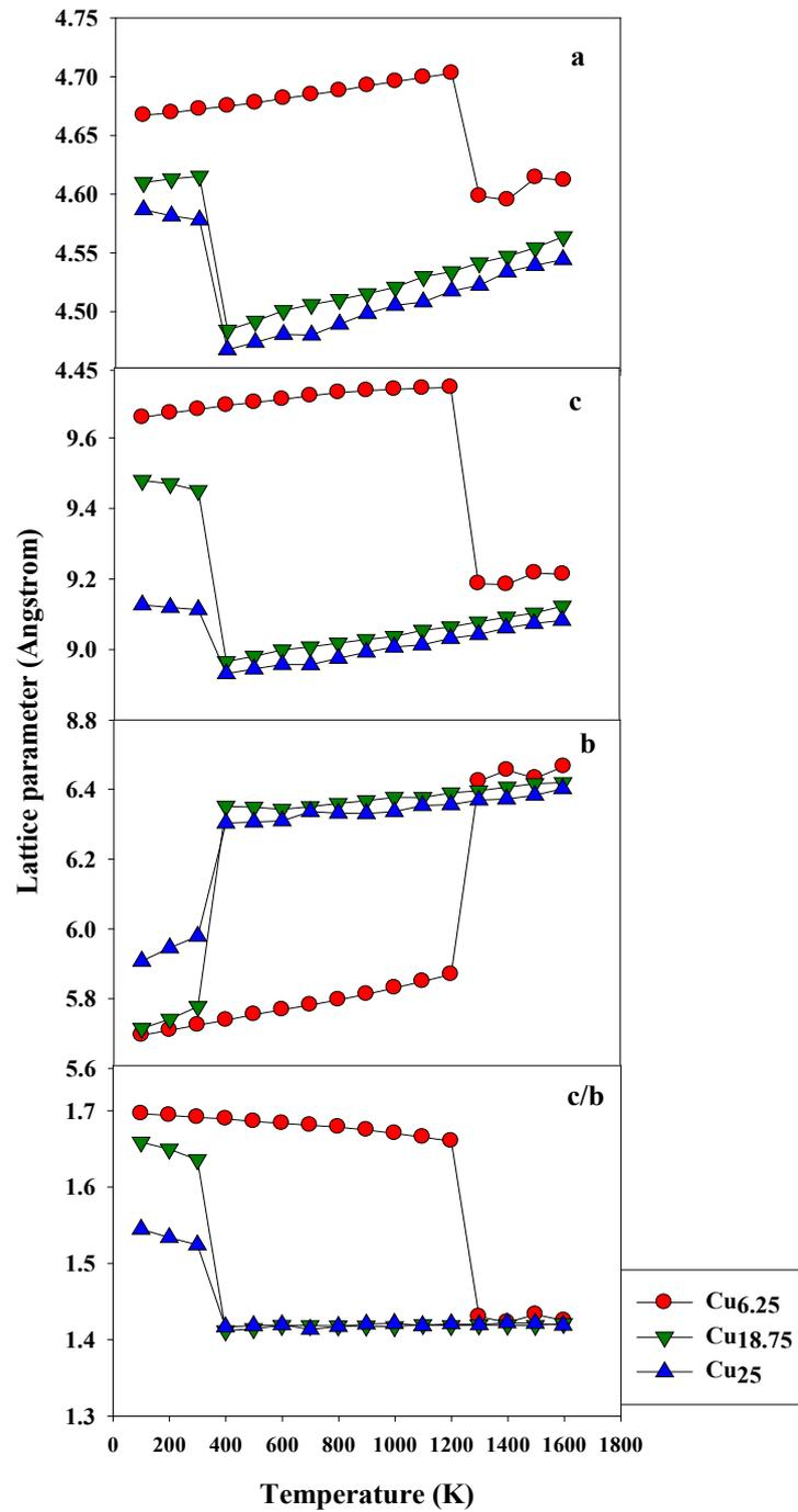
**Figure 2.** The effect of temperature on the a, c, b and c/b lattice parameters of the B19 TiPt and  $Ti_{50}Pt_{50-x}Cu_x$  ( $x = 6.25, 18.75$  and 25)
