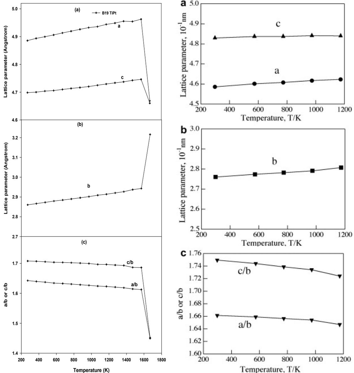
**Figure 1:** The effect of temperature on the *a*, *c*, *b*, *c/b* and *a/b* lattice parameters of the B19 TiPt on the left hand side compared with the experimental results [14] on the right hand side
