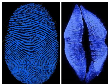
Fig. 2: Fingerprint and lip print developed using the synthesized nanophosphor excited under UV light.
