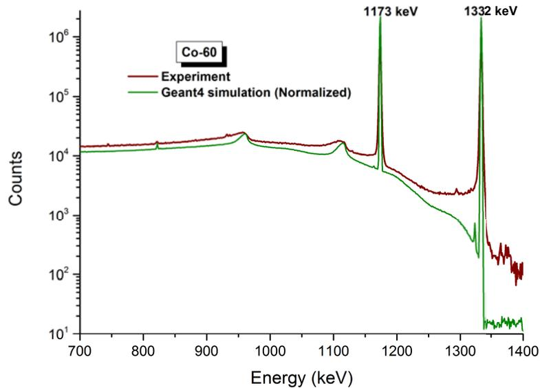
**Figure 4.** Comparison of the simulated and experimental gamma spectra from  $^{60}\text{Co}$  for the AFRODITE clover detector system. The green line shows the simulated spectrum and red line shows the experimental spectrum. Normalization was done according to the number of gammas emitted by the source in the experiment and number of gamma histories in the simulation.
