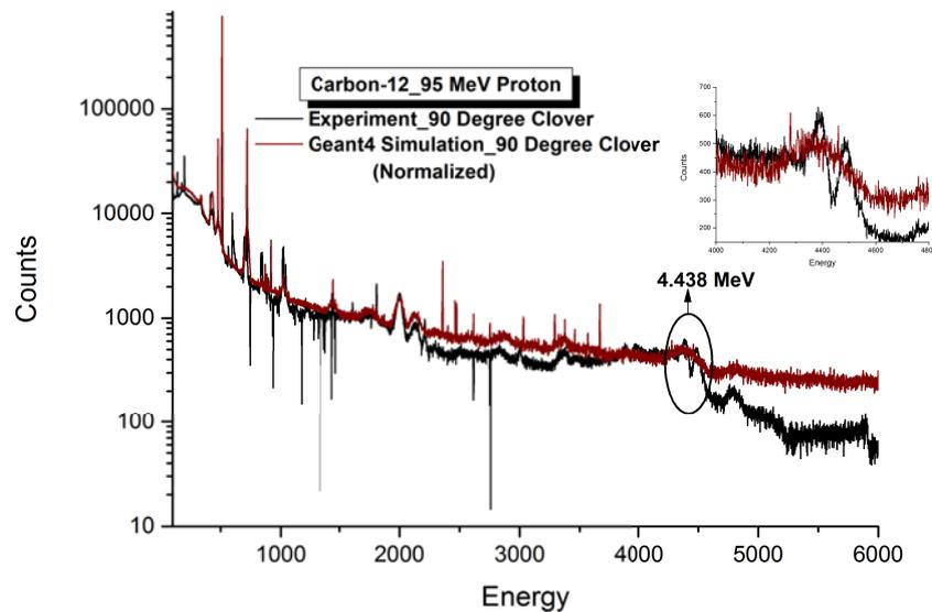
**Figure 5.** Gamma spectra comparison of the experimental and simulated results for a 95 MeV proton collision on the carbon target. The red line shows the corrected Geant4 simulated spectrum and the black line shows the experimental spectrum. Inset: Enlarged view of the 4.438 MeV gamma peak. Normalization was done according to the difference in the number of incident protons, the difference in the target thickness and the absolute detector efficiency correction factor.
