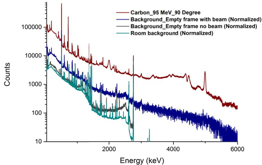
**Figure 3.** The red line shows the raw data for the 95 MeV proton bombardment of the carbon target, cyan color line is room background, the blue line indicates the background radiation from the frame with the beam on, and the gray line shows the background from the target frame with the beam off. These spectra were measured by the clovers placed at 90 degrees to the beam line. Normalization was done according to the time acquisition and the integrated proton charge.
