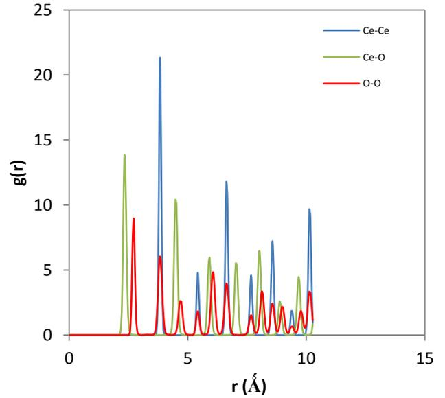
Figure 2. The radial distribution functions of an O vacancy in fluorite CeO<sub>2</sub> supercell at 300 K.
