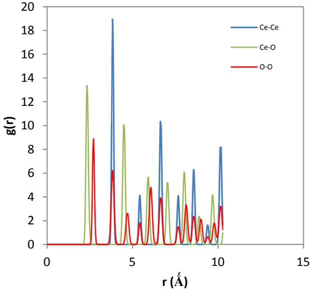
Figure 1. The radial distribution functions of fluorite CeO<sub>2</sub> supercell at 300 K.
