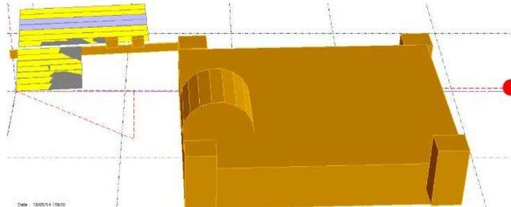
**Figure 2.** PVsyst 3D scene of shading on 18 May 15:30h as viewed from the North. The building in the foreground is casting shadow on the PV system in the background.
