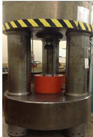
**Figure 2.** The frame of the force comparator machine.
