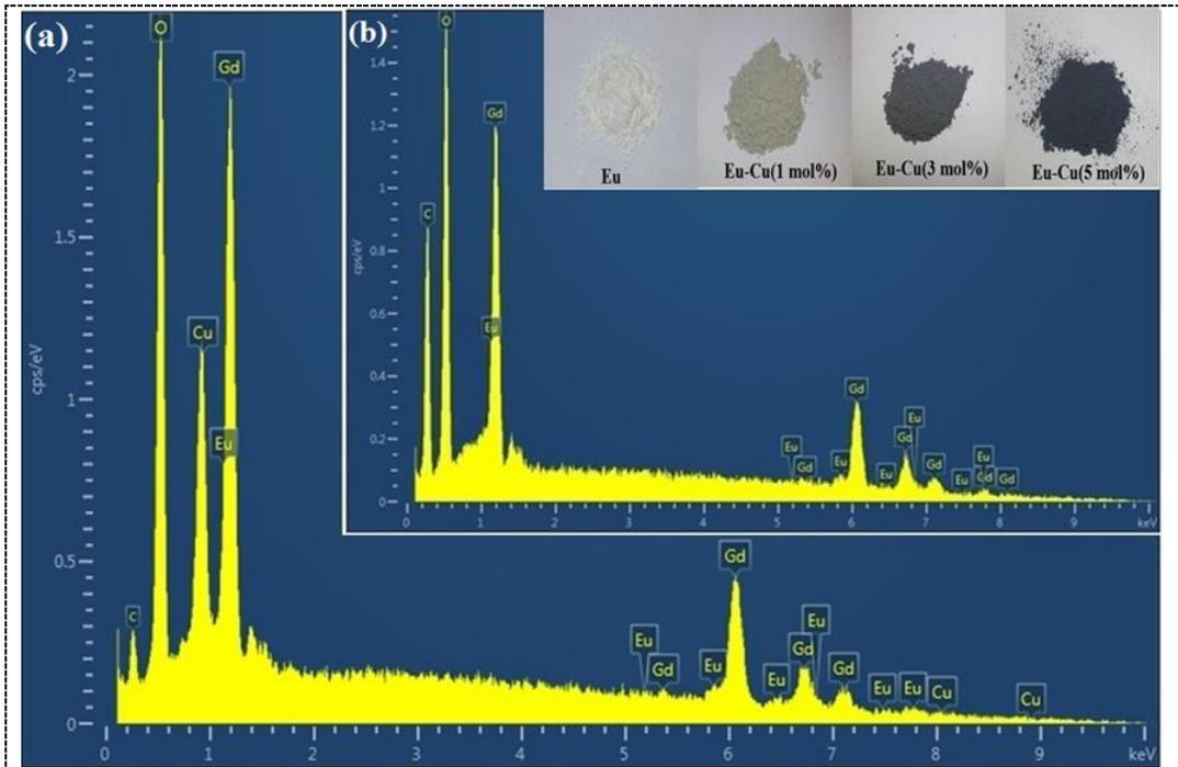
**Figure 3.** EDS images of the Gd<sub>2</sub>O<sub>3</sub>:Eu with (a) CuO and (b) without CuO nanosheets with their optical photographs as indicated.
