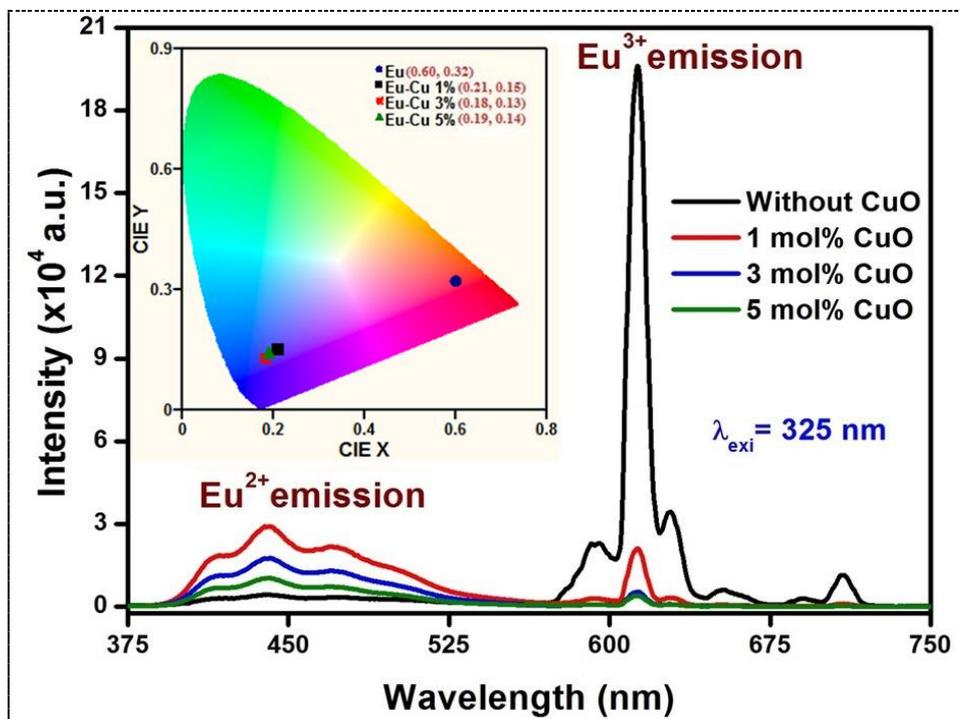
**Figure 4.** PL emission spectra of the Gd<sub>2</sub>O<sub>3</sub>:Eu nanosheets with different CuO concentration and corresponding colour coordinates (inset).
