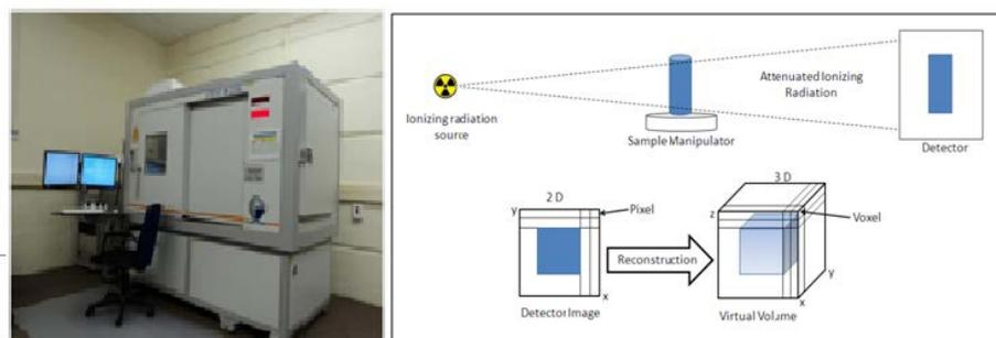
**Figure 2:** Micro-focus X-ray machine and tomographic process at the MIXRAD facility at Necsa
