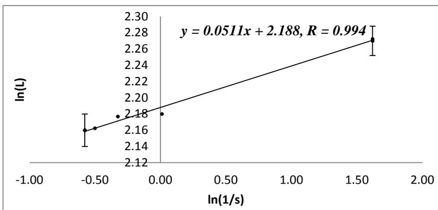
**Figure 6:** Ln-Ln fractal analysis plot for the large brick sample
