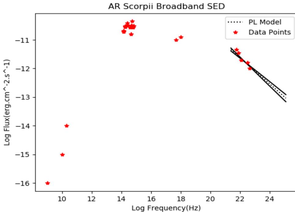
**Figure 8.** Proposed Broadband SED of AR Sco, ranging from radio to gamma-ray energies. Radio and optical data adapted from Marsh et al.<sup>[1]</sup> and Geng et al.<sup>[2]</sup>. The dashed and solid lines show the Power Law model butterfly plot produced by the Likelihood Analyses generated in Fermipy.
