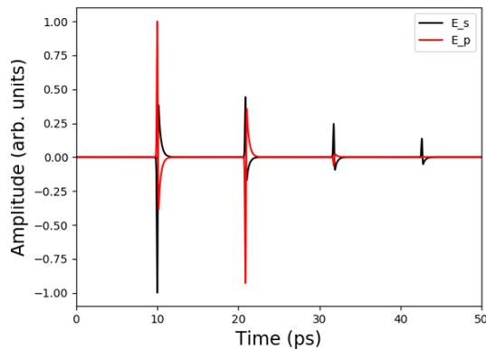
**Figure 7.** Normalized time-domain electric fields generated by taking an IFFT of electric fields presented in figure 5.
