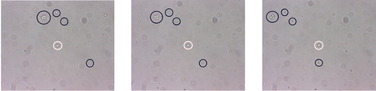
Figure 4. This figure shows the movement of a trapped 1 \mu\text{m} bead (circled in white) relative to the other freely diffusing 1 \mu\text{m} beads (circled in black). This is achieved by moving the sample to the left while the trap position remains stationary.
