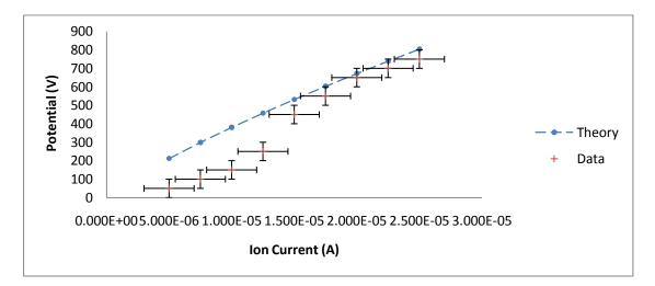
Figure 2. Comparison of data with model for the electrical behavior of the thrusters.
