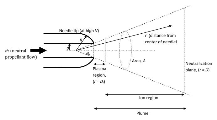
**Figure 1**. Schematic of the exhaust plume. The neutral propellant exits through the needle into vacuum, giving rise to an expanding cone of gas.
