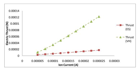
Figure 3. Comparison of the vector heating (VH) and electrostatic (ES) thrust models.
