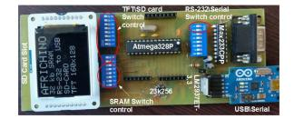
**Figure 2.** Overview of the entire board. The USB-Serial converter is an Arduino device. The USB to Serial converter is indicated on the board as USB\Serial. The red circles indicates the switch-dip to activate or deactivate the different parts of the Board.
