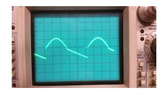
**Figure 4.** The curve generated by Africhino following the concept of Direct Digital Synthesis (DDS) [7].
