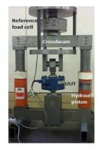
**Figure 6.** Calibration set up of force transducer in tension.
