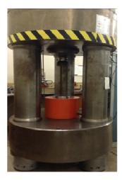
**Figure 1.** A schematic diagram of the frame of the force comparator machine.
