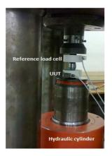
**Figure 5.** Calibration set up of force transducer in compression.
