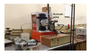
**Figure 4.** The hydraulic system consisting of the hydraulic pump and a stepper motor coupled to a Budenberg pressure balance.
