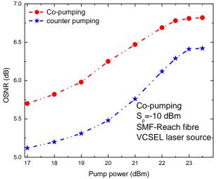
Figure 2: OSNR variation with pump power for co-pumping and counter pumping schemes of a 25 km ITU-T G.655 fibre.
