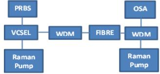
Figure 1: Raman amplified optical transmission
