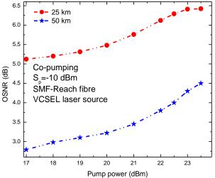
Fig 3 shows the OSNR performance of a 25 km and 50 km ITU-T G.655 fibre lengths at co-pumping scheme.
