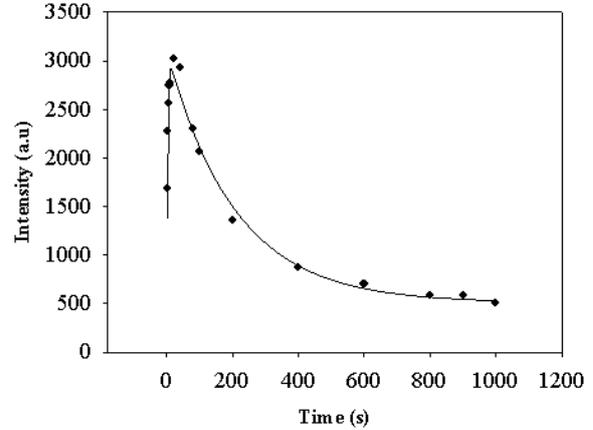
**Figure 3.** Variation of PTTL intensity with illumination time.
