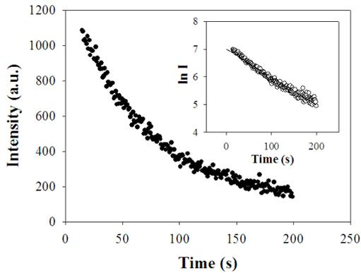
**Figure 4.** Phosphorescence measured at 55°C following a 200 Gy dose. The inset shows a semi-log plot of the intensity against time.
