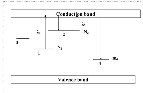
**Figure 9.** Energy band diagram to explain PTTL.
