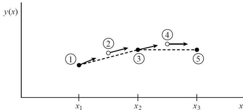
Figure 2: The 2nd Order R-K, or the Midpoint method. Second-order accuracy is obtained by using the initial derivative each step to find a point halfway across the interval, then using the midpoint derivative across the full width of the interval. In the figure, filled dots represent final function values, while open dots represent function values that are discarded once their derivatives have been calculated and used. (Numerical Recipes Figure 16.1.2.)
