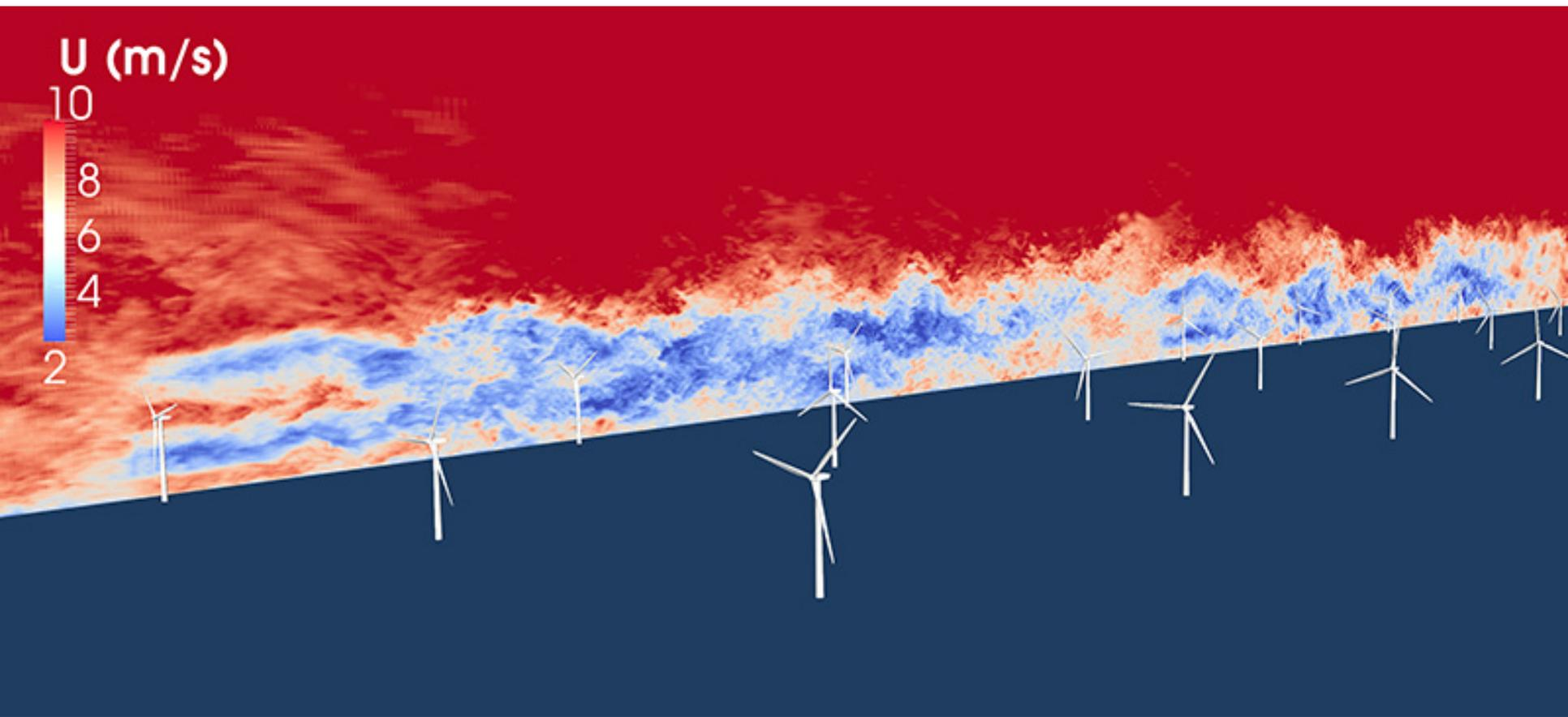
This computer-generated simulation shows the turbulent nature of wind turbine wakes. The simulation helped uncover potential differences in output between downstream 'waked' turbines and upstream turbines.
