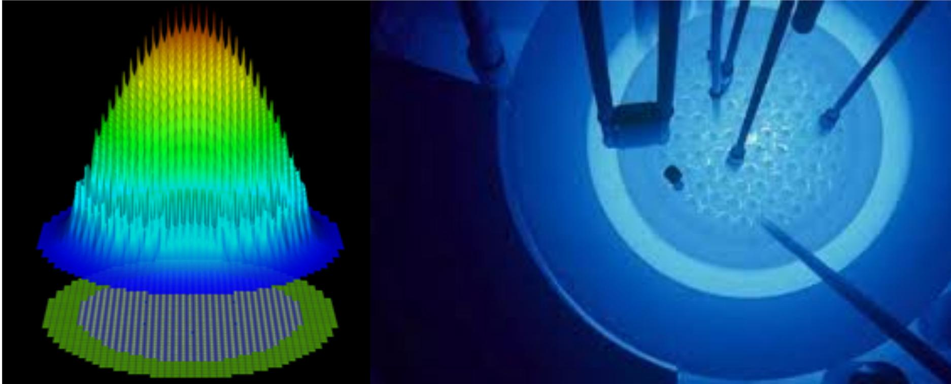
An elevation plot of the highest energy neutron flux distributions from an axial slice of a nuclear reactor core is shown superimposed over the same slice of the underlying geometry. This figure shows the rapid spatial variation in the high energy neutron distribution between within each plate along with the more slowly varying, global distribution. UNIC allows researchers to capture both of these effects simultaneously. (Courtesy: [Argonne National Lab/Flickr](#))
