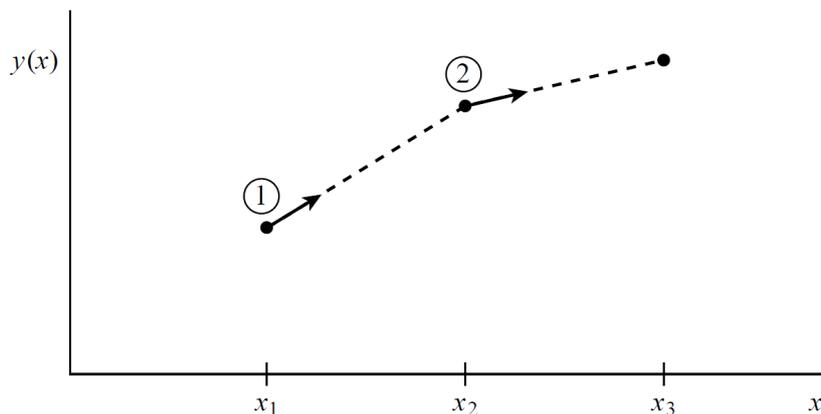
Figure 1: Eulers method. In this simplest (and least accurate) method for integrating an ODE, the derivative at the starting point of each interval is extrapolated to find the next function value. The method has first-order accuracy. (Numerical Recipes Figure 16.1.1.)
