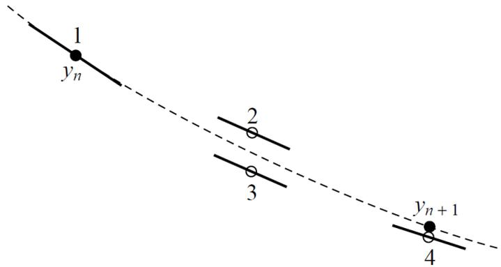
Figure 3: Fourth-order Runge-Kutta method. In each step the derivative is evaluated four times: once at the initial point, twice at trial midpoints, and once at a trial endpoint. From these derivatives the final function value (shown as a filled dot) is calculated. (Numerical Recipes Figure 16.1.3.)
