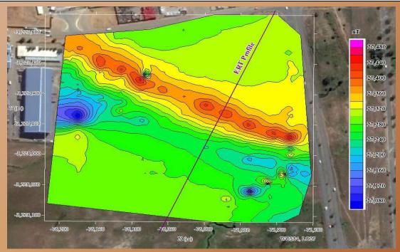
Contour map of the total magnetic field recorded across the edge of a suspected ring-dyke.
