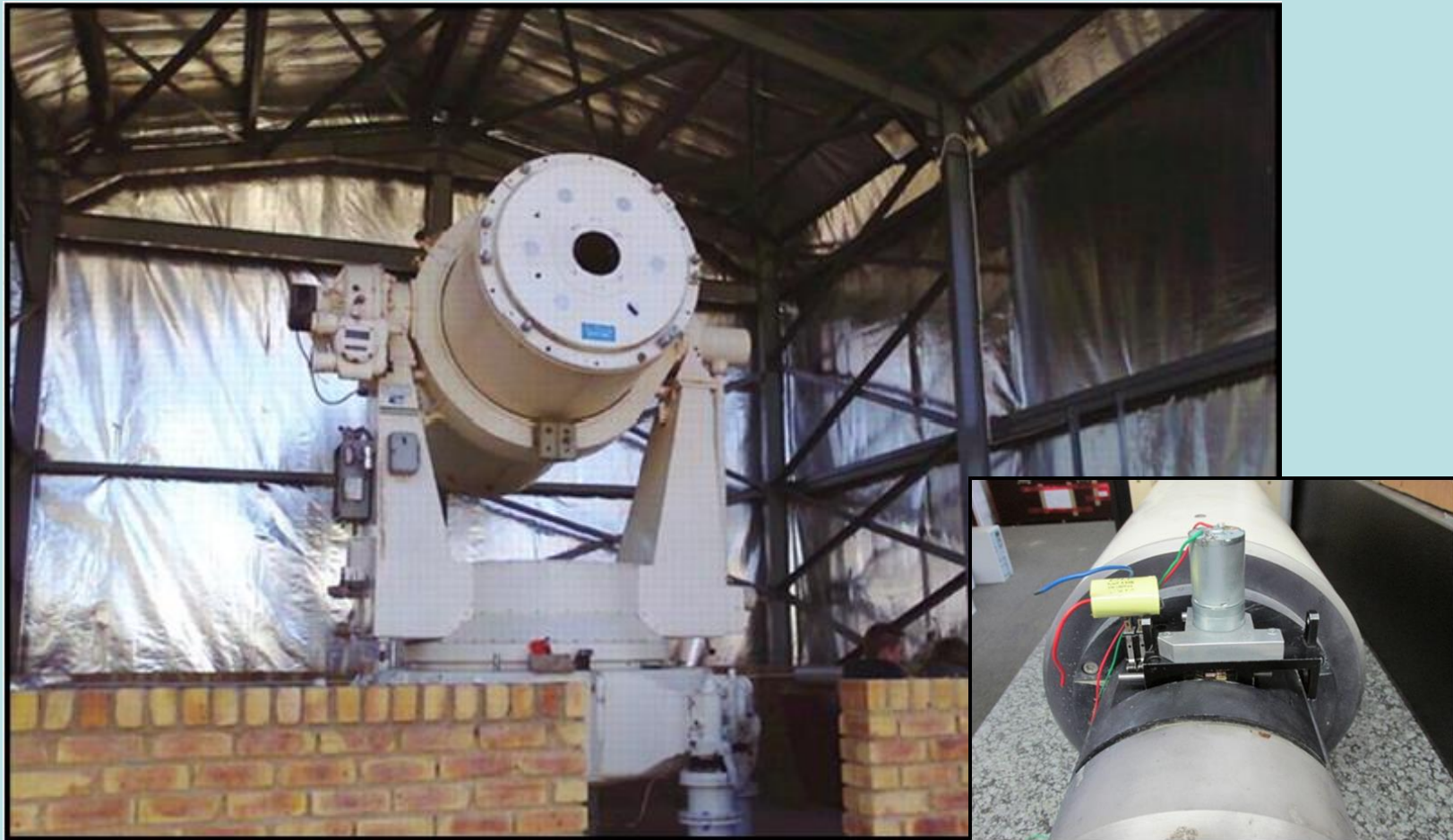
Figure 2: The ex-OCA 1 m telescope installed on its foundation at HartRAO and the new assembly of the DC motor to control the objective lens of the beam expander.
