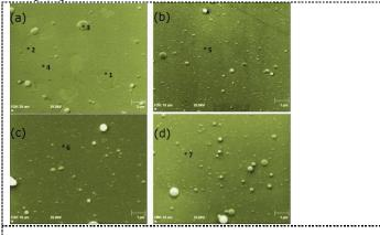
**Figure 3.** SEM images, for the thin film surfaces, grown in (a) base, (b)  $O_2$ , (c) Ar and (d)  $N_2$  pressure.
