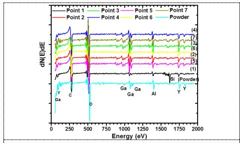
**Figure 4.** Different AES spectra of Y<sub>3</sub>(Al,Ga)<sub>5</sub>O<sub>12</sub>:Tb powder (a) and thin films grown in base pressure (b-e), (f) O<sub>2</sub>, (g)Ar and (i) N<sub>2</sub> atmospheres.
