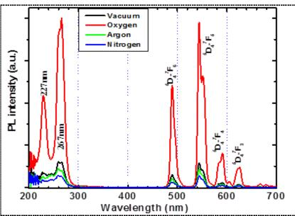
**Figure 7.** PL emission and excitation of Y<sub>3</sub>(Al,Ga)<sub>5</sub>O<sub>12</sub>:Tb thin films grown in different working atmosphere (Excitation measured at an emission wavelength of 544 nm; emission measured at an excitation wavelength of 267 nm).
