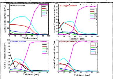
**Figure 5.** Depth profiles of the thin films structures, that were grown in (a) base, (b)  $O_2$ , (c) Ar and (d)  $N_2$  atmospheres.
