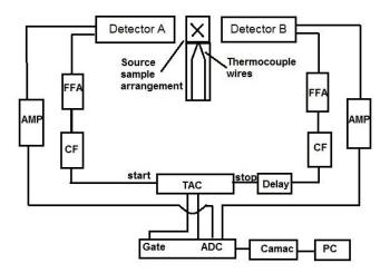
**Figure 1.** Setup used for positron annihilation investigation. Circuit diagram shows a two-detector system that was used. The two detectors measured the electron-positron annihilation radiation  $(511 \pm \Delta E)$  KeV at defects and in bulk.
