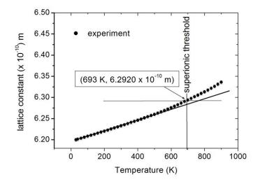
**Figure 3**. Variation of lattice constant in BaF<sub>2</sub> as a function of temperature.
