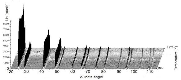
Figure 2. Measured X-ray diffraction patterns in  $BaF_2$  in the temperature range 300 - 1173 K.
