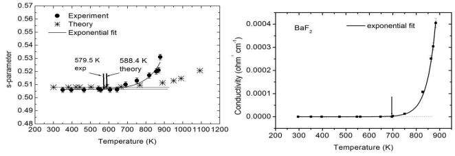
**Figure 6**. Comparison between theoretically and experimentally determined s-parameters. The experimental large deviation of which begins at ~579.5 K compares well with a theoretically calculated deviation.
