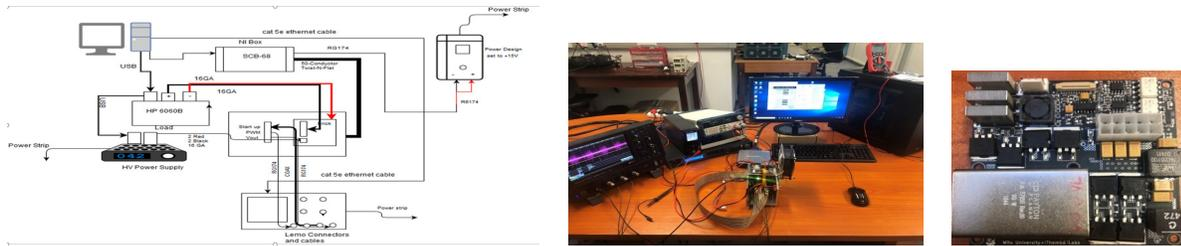
**Figure 5.** Functional block diagram of the LVPS test station (left), Test station setup at Wits (middle), and LVPS prototype manufactured in South Africa (right).
