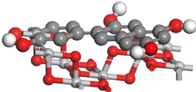
**Figure 5:** Structure of Cyanidin dye molecule adsorbed on TiO<sub>2</sub> anatase (100) surface
