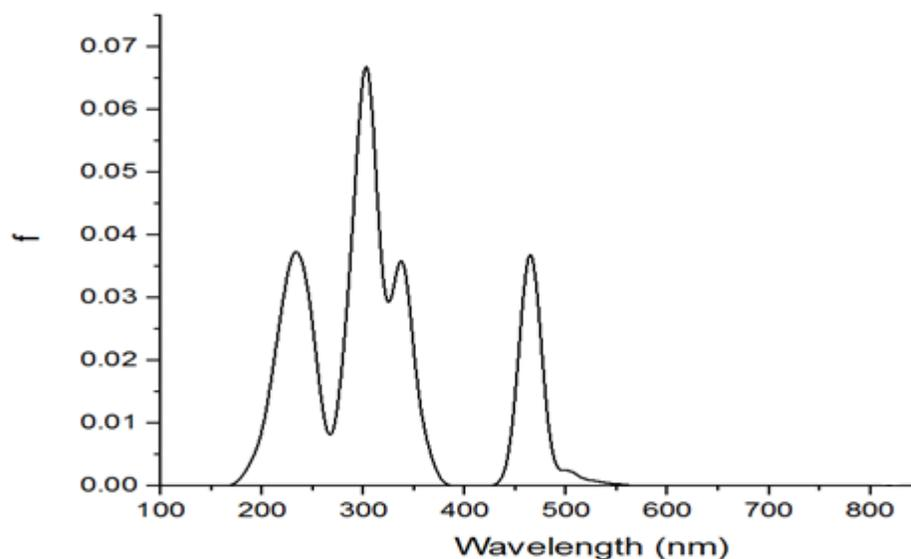
**Figure 4:** Calculated UV-Vis spectrum for cyanidin dye molecule
