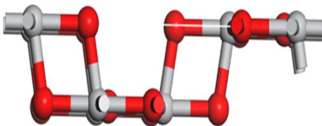
**Figure 1:** Structure of TiO<sub>2</sub> anatase (100) surface, red represent oxygen and grey represent titanium. Figure 1 illustrate the structure of TiO<sub>2</sub> anatase (100) surfaces cleaved from anatase TiO<sub>2</sub> bulk structure. The atoms in this surface are having some cleaved bonds in the termination position, while terminating with both oxygen and titanium. The surfaces were optimized by relaxing atoms to eliminate surface tension.
